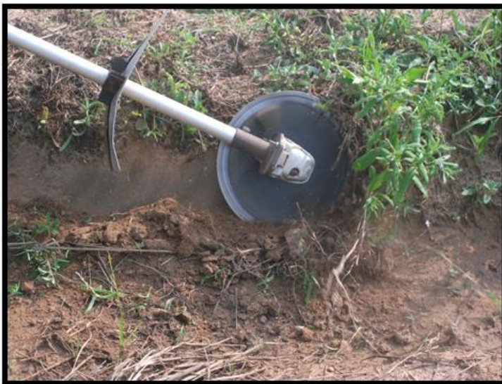
Fig.6. Performance evaluation of trimming of bund in dry land
