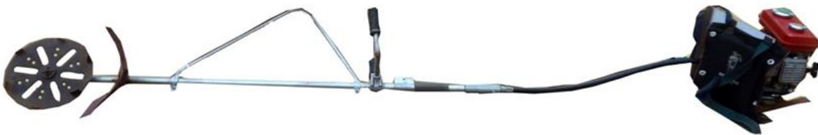
Fig. 1. Development of Engine Operated Bund Trimmer
