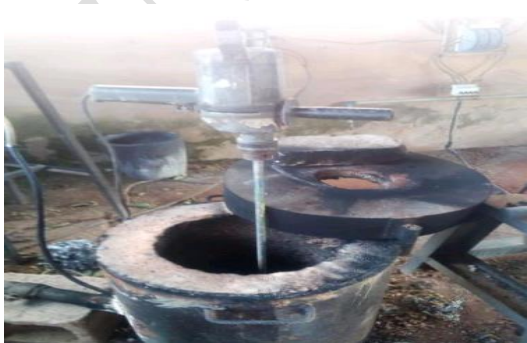
Fig. 6: Mechanical Stirring with furnace
