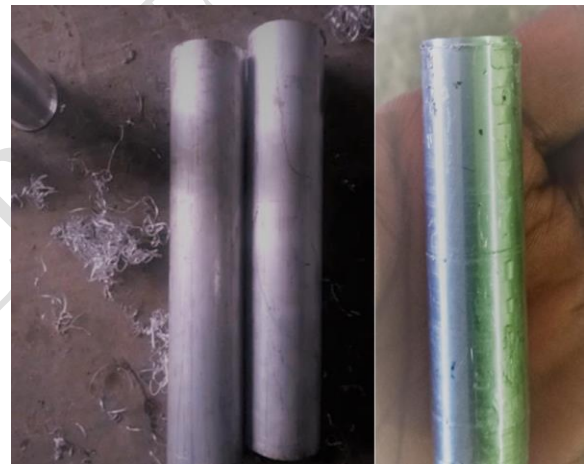
Fig. 9: Al. A6351 Egg-shell machined sample
