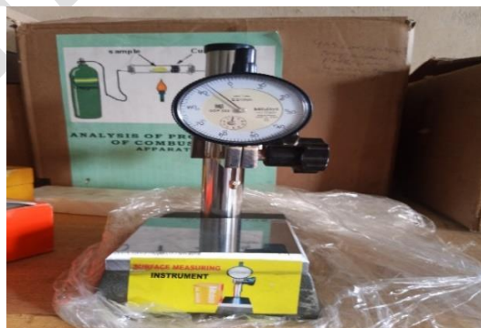
Fig. 5: Mutotuyo surface measuring instrument
