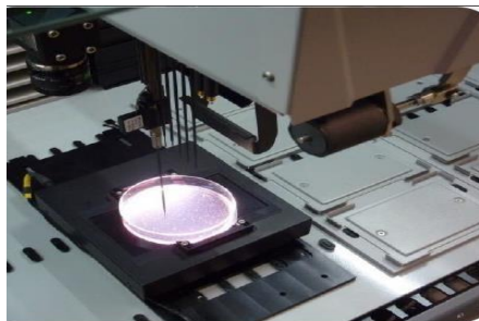
206 Fig 5: PickoCell™ picking stem-cell colonies on Tecan Robots
