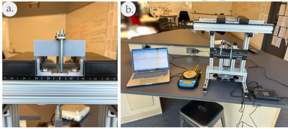
Fig.4a) Example of test model loaded into the VSMT for data-gathering Fig.4b ) View of the experimental set up, displaying [left to right] computer with google slides to record model weights, scale to measure model weights, Vernier Structures and Materials Tester to measure model load capacity and displacement, Labquest 2 to record VSMT data and transfer to computer via internet
