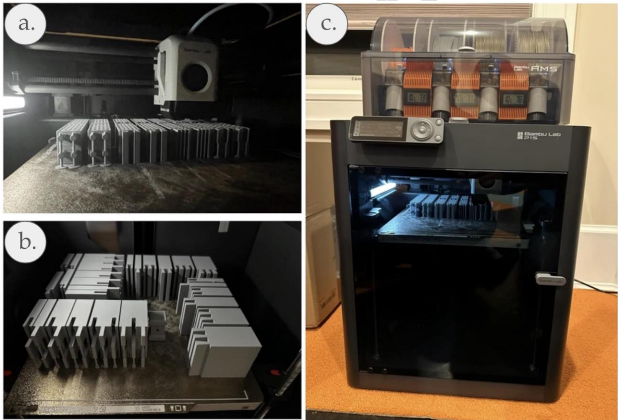
Fig.2: Bambu Lab P1S printer used in the experiment Fig.2a) Inside of printer midway through printing models Fig.2b) Models on build plate after finishing print Fig.2c) Bambu Lab P1S used to print the models
