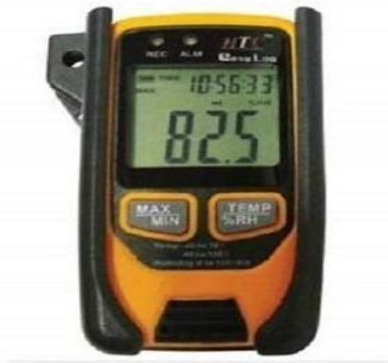
Plate 6: Data logger used for monitoring environmental data inside the polyhouse
