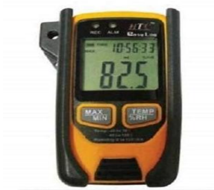
Plate 4: Data logger used for monitoring environmental data inside the polyhouse
