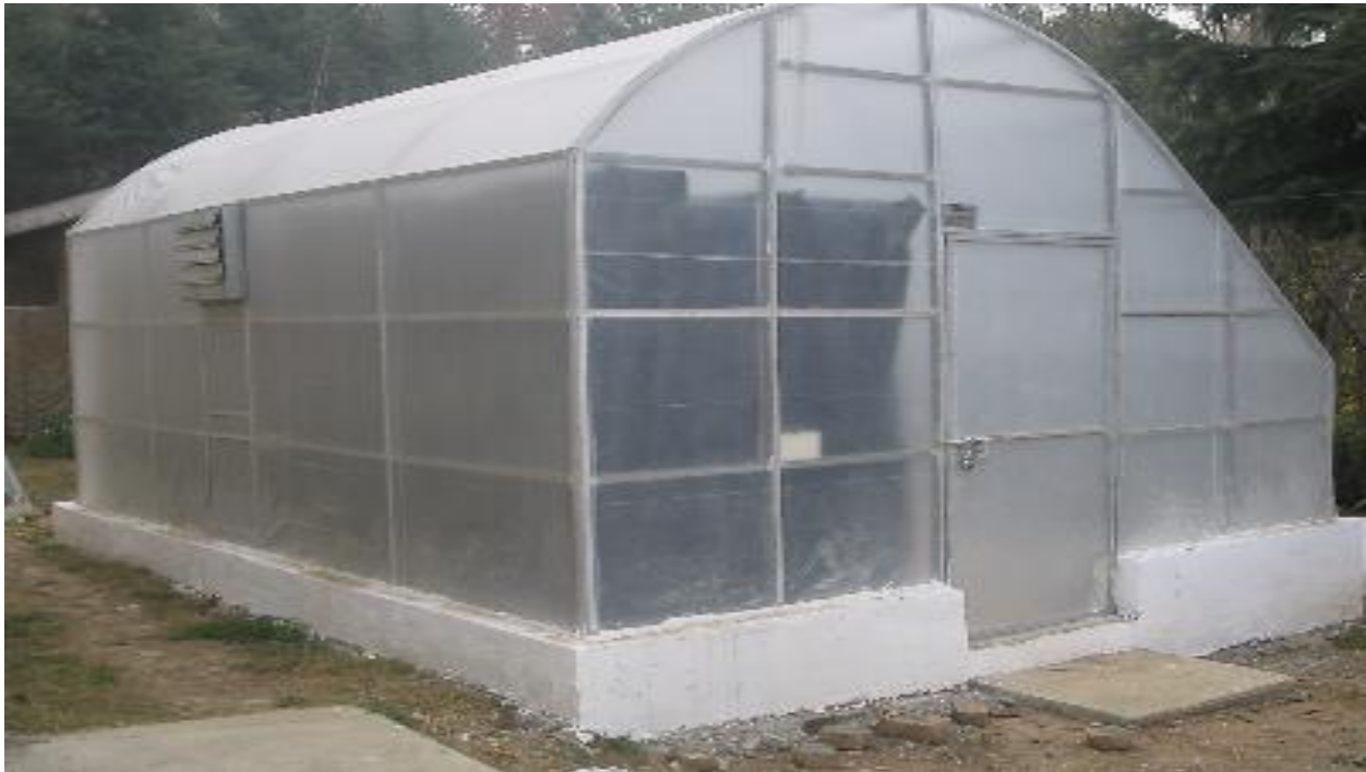
Plate 1: Greenhouse type solar multi-tier tunnel dryer
